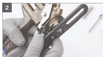
2 Tighten fluid tip by hand using the universal spanner.
