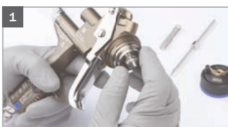
1 Assembly of the fluid tip
