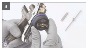
3 Assembly of the air cap
