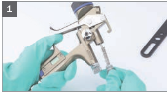
1 First remove paint needle.
