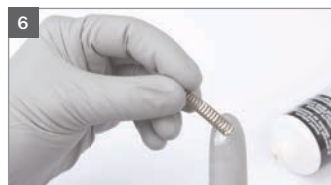
6 Grease and insert paint needle spring
