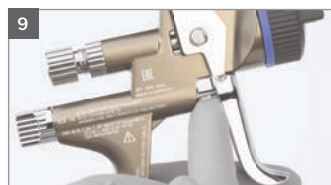
9 Grease visible part of air piston rod
